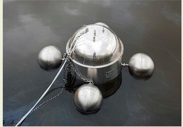
Measurement of greenhouse gas emissions from tailings basin and mine area.
